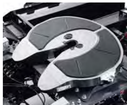
ALUMINIUM FIFTH WHEEL reducing vehicle weight by 22 kg.
