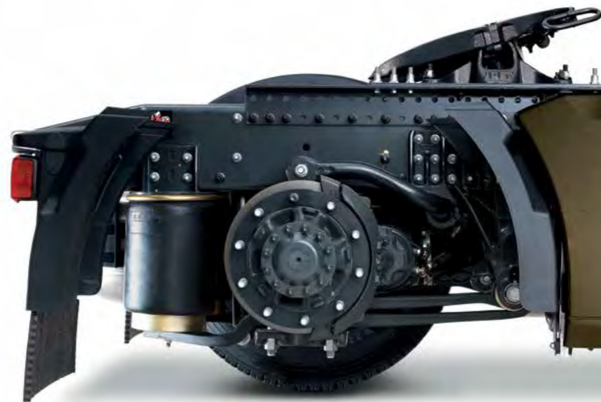
REAR AIR SUSPENSION design capacity 13 t.
