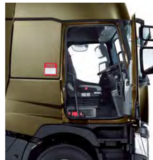
DOOR OPENING ANGLE 85° for easier cab access.
