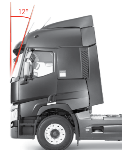
12° INCLINED WINDSCREEN for a better aerodynamic profile.
