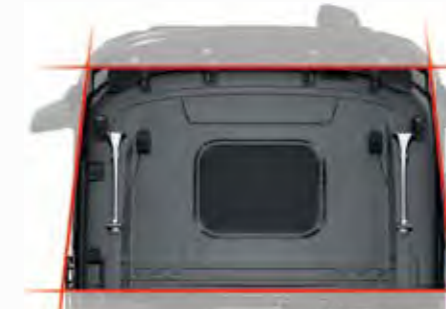
TRAPEZOID-SHAPED CAB 2.3 metres at the front and 2.5 metres at the rear to improve air flow.
