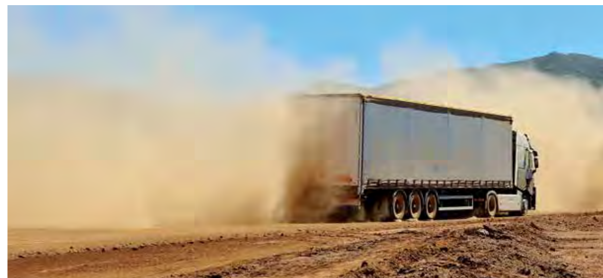
EXTREME TEMPERATURE TEST in Almeria, Spain to measure vehicle resistance to harsh conditions (dust, heat, etc.).
