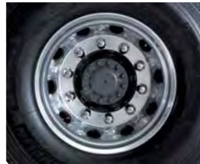
ALUMINIUM WHEELS reduce vehicle weight by up to 160 kg on 6x2.
