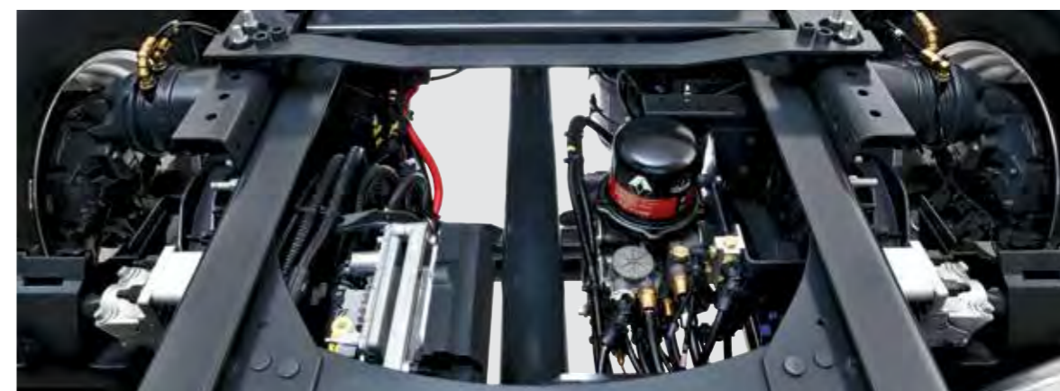
SEPARATION OF WIRING HARNESSES AND AIR PIPES for easier maintenance.
