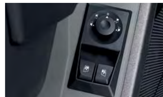
MANAGEMENT OF REARVIEW MIRRORS AND WINDOWS one-touch window lift and electrical adjustments for main and wide angle rearview mirrors*.
