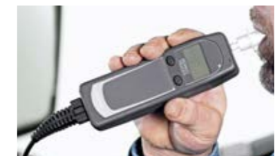
BREATHALYZER IGNITION INTERLOCK lets drivers check blood alcohol level before starting the vehicle.
