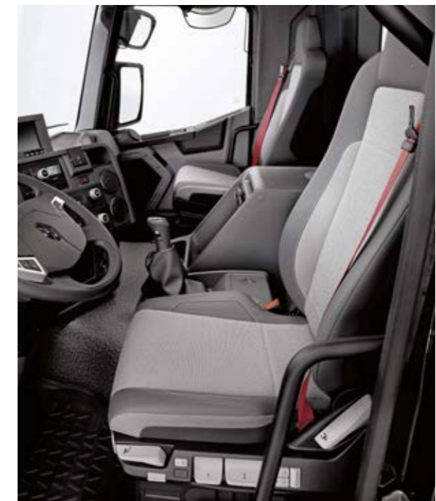
VENTILATED, HEATED, AIR-SUSPENDED SEATS with on-board seat belts, headrests, side and lumbar support adjustment, backward movement range 20 cm.
