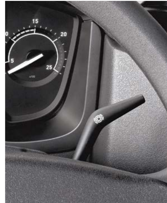
RETARDER CONTROL Optibrake, Optibrake+ and Voith.
