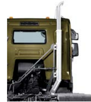
VERTICAL OUTLET for better body mounting options.
