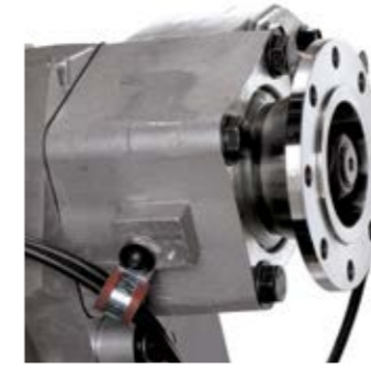
POWER TAKE-OFF for operating bodybuilder mounted equipment when moving or stationary.
