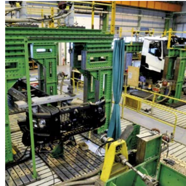
VIBRATION TEST BENCHES with thousands of hours of testing to safeguard cab reliability.
