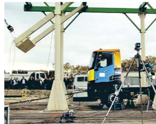
FRONTAL IMPACT to measure the cab's resistance to impact.
