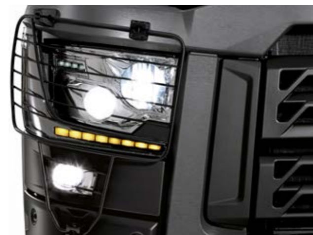
HEADLAMP PROTECTION GRILLES and polycarbonate headlamps as standard for better impact resistance.
