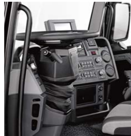
POSITION FOR ENTERING/ LEAVING THE VEHICLE to make driving position access easier.
