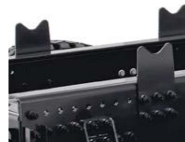
PLATED MOUNTING BRACKETS ON SIDE MEMBERS for easier body mounting.
