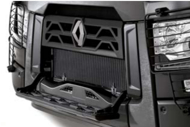
WINDSCREEN ACCESS STEPS non-slip to make servicing the vehicle easier.
