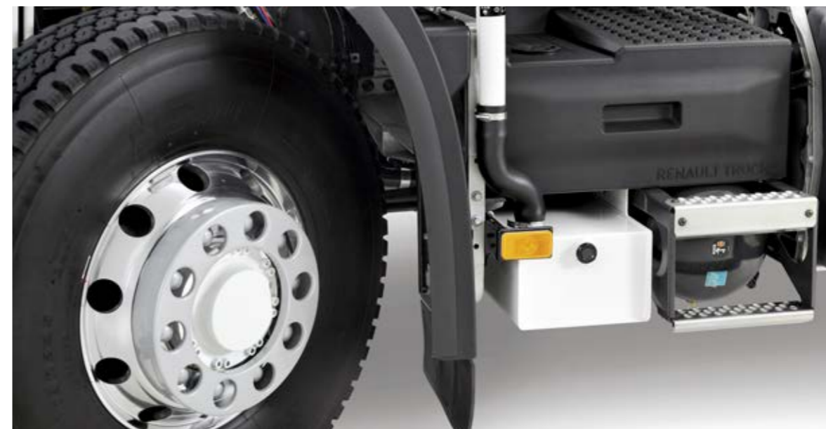
OIL RESERVOIR INSTALLED UNDERNEATH THE BATTERY BOX to free up more available space on the chassis.
