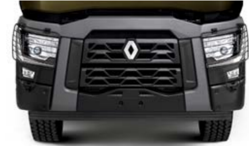
BUMPER WITH STEEL CORNERS for combined use (as standard).
