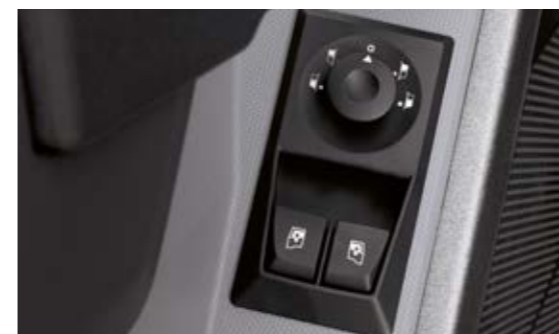
ONE-TOUCH CONTROL OF SIDE WINDOWS AND MIRRORS and electrical adjustment of main and wide angle rearview mirrors.
