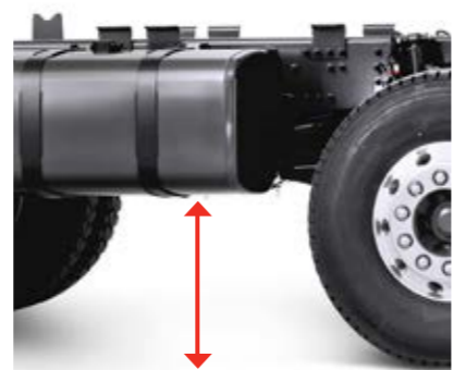
GROUND CLEARANCE UNDER TANK 440 MM*
