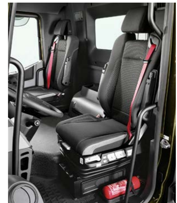
HEATED AND VENTILATED SUSPENDED SEATS with integrated seat belts, headrests, lumbar and side support adjustment, plus 20 cm movement for more leg room.
