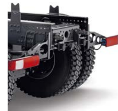
REAR OVERHANG available in increments of 50 mm to avoid re-cutting the side members.
