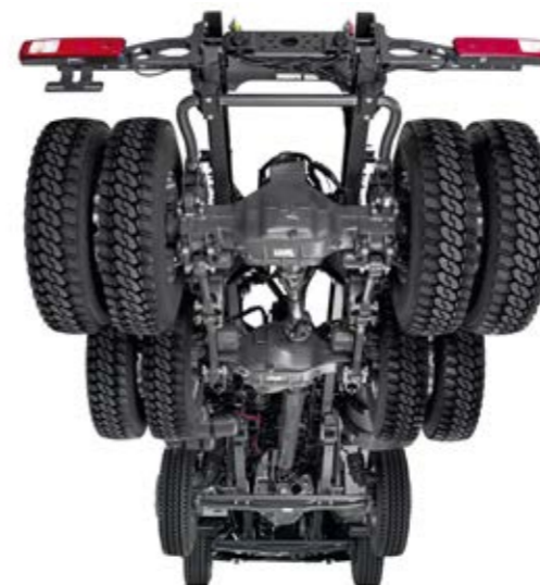
DOUBLE REDUCTION TANDEM DRIVE AXLE for greater traction on difficult terrain.
