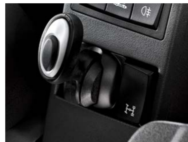
SYSTEM ACTIVATED AND DEACTIVATED FROM THE DASHBOARD by means of a single button at speeds of between 0 and 25 km/h.
