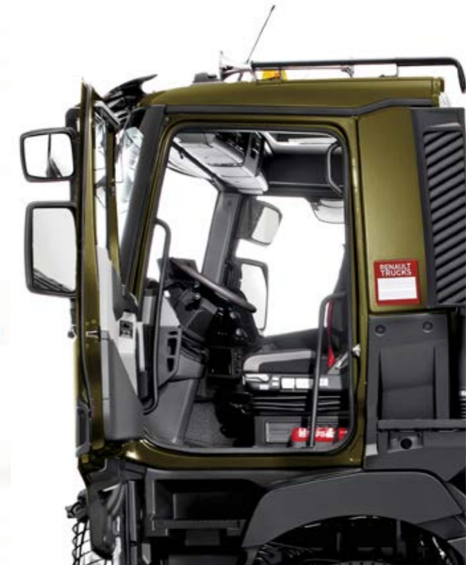
DOOR OPENING ANGLE 85° for easier cab access.
