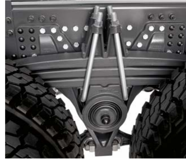
MECHANICAL OR AIR REAR SUSPENSION 21 t parabolic, 3 leaf springs, 26 t parabolic, 3 leaf springs, 21 t 2x2 cushions or 26 t 2x4 cushions.
