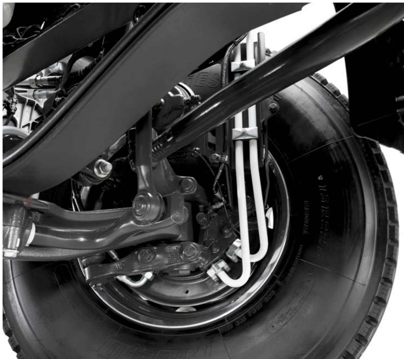
FRONT AXLE EQUIPPED WITH TWO HYDRAULIC MOTORS with a unit power rating of 41 kW.
